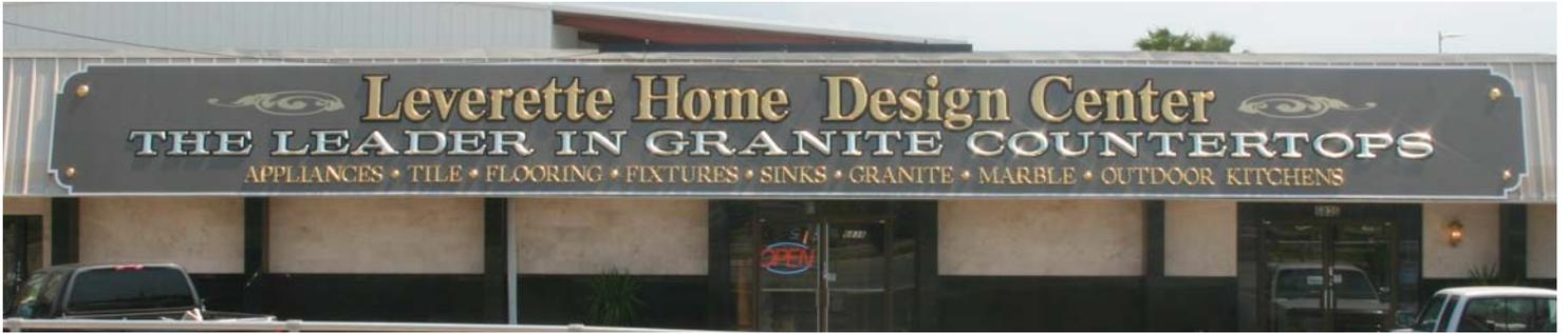
The main copy is 24-in. Times letters from Gemini, with 12-in. Times Extended for *The Leader*. . . The list across the bottom is 8-in. lettering. Overall, the sign is 6-by-64-ft, with a background of PVC sheet painted with automotive paint. "That's the biggest single gold leaf letter sign we've done," says Mike.
